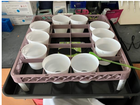
Figure 25. Image of Hatchery System Setup for Year 2. The hatchery system consists of a tray of 10 cups with mesh bottoms in a water bath with a heater and bubble filter. The cups are labeled with
