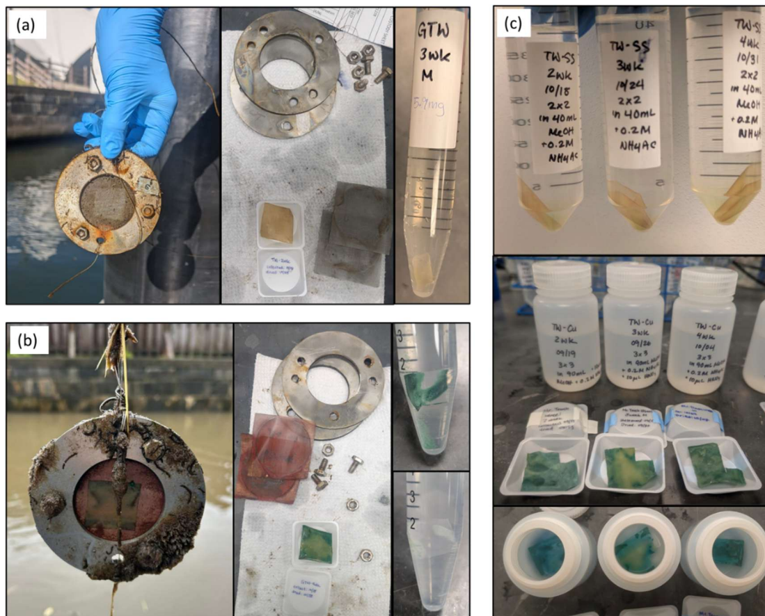
Figure 3.4. Passive sampler retrieval and processing. After retrieval, the passive samplers were cleaned and disassembled. Samplers with protective (a) stainless-steel mesh required less processing compared to the those using (b) copper mesh due to the absence of copper scale formed on the membrane during deployment. (c) MeOH digestion of 2 \times 2 \text{ cm}^2 and 3 \times 3 \text{ cm}^2 membrane coupons removed from the passive samplers with protective stainless-steel and copper meshes, respectively.
