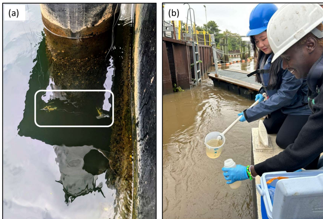
Figure 3.3. Sample deployment and retrieval. (a) Passive samplers were tied to semi-permanent structures with stainless steel wire and nylon fishing line. Both options were used as a fail-safe in case either line was cut during deployments. (b) 500-mL grab samples (duplicate) were collected during passive sampler deployment and retrieval.
